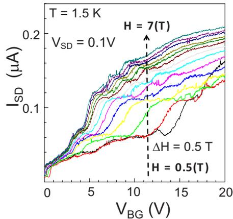
FIG. 3. (Color online)  $I_{SD}$  at  $T=1.5$  K as a function of  $V_{BG}$  for various magnetic fields applied perpendicular to the tube longitudinal axis.
