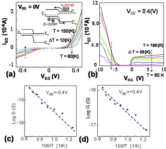
FIG. 2. (Color online)  $I_{SD}$  as functions of (a)  $V_{SD}$  and (b)  $V_{BG}$  for various temperatures. Dotted line in (a) is a calculation result based on Eqs. (1) and (2). Insets of (a): schematic views of band structures in forward (+) and reverse (-)  $V_{SD}$  regions (right and left, respectively). [(c) and (d)] Thermal-activation-type relationship in conductance ( $G$ ) vs temperature at  $\pm V_{SD} = 0.4$  V in (a).
