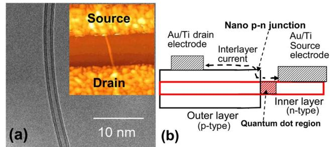
FIG. 1. (Color online) (a) TEM image of DWNT. Inset: AFM images of isolated one DWNT located between source (S) and drain (D) electrodes with 800 nm spacing in a FET. (b) Schematic cross section of the FET with electrode contacts to different layers.
